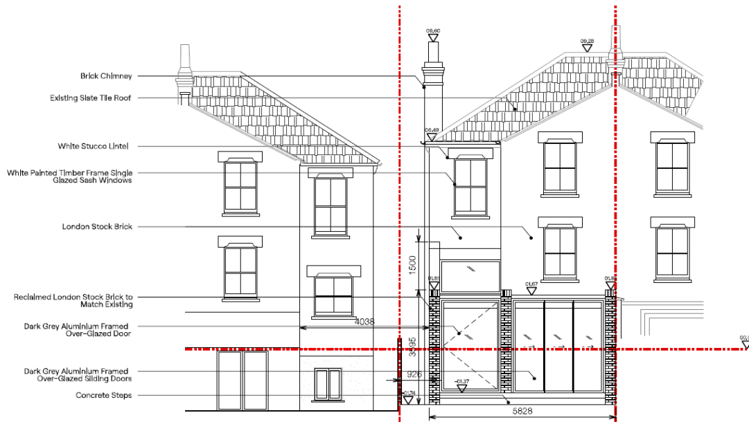
Figure 3: Proposed rear elevation
